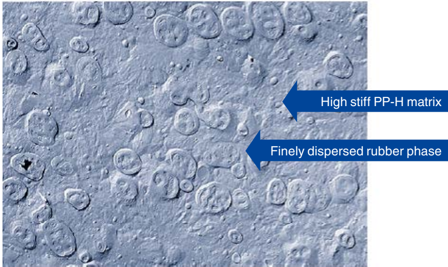
Figure 2. Morphology of HM PP-B copolymer [2] .
