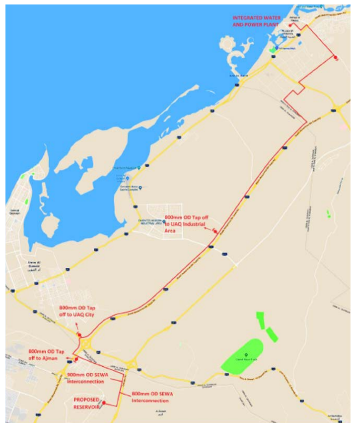
Figure 8. Map of the UTICO Ras Al Khaimah to Sharjah 1200 and 1400mm OD Water Pipeline.
