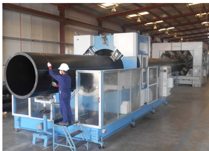
The 1200mm OD pipeline being produced at the UTICO manufacturing facility.
