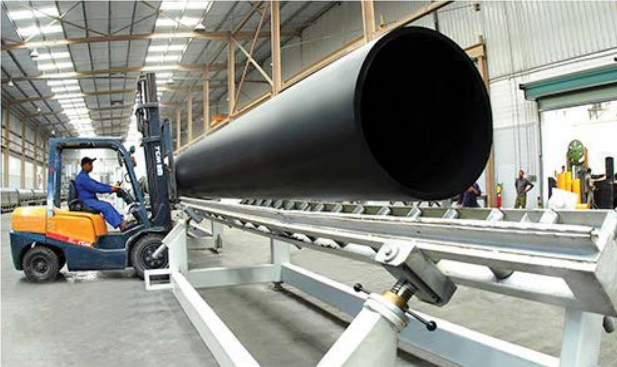
Large diameter PE100 pipes being produced at Gulf Manufacturing Company.
