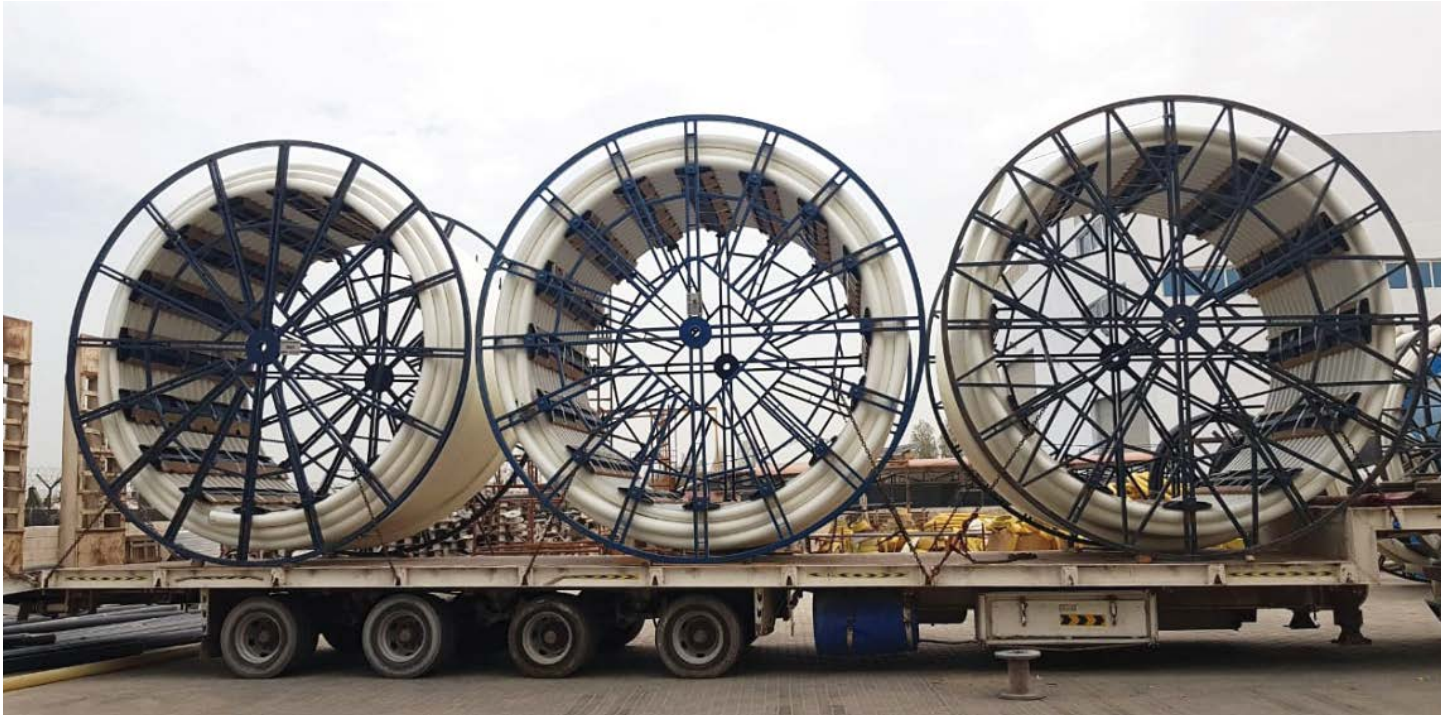
The project was delivered by low-bed trailers that could fit up to 1.2km of RTP pipes per trailer.
