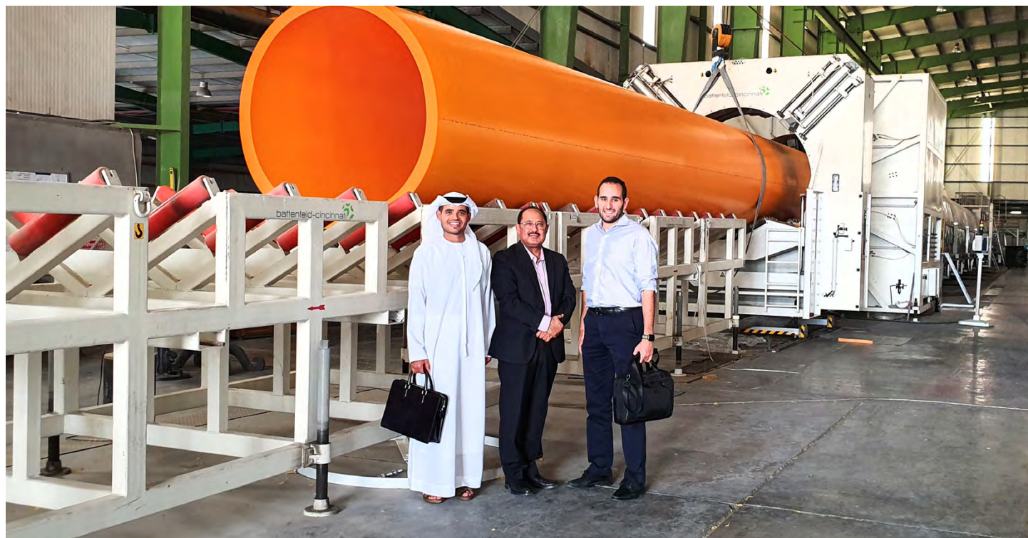
A SDR21 1600mm OD PE100 being produced in UPI for a North American project.
