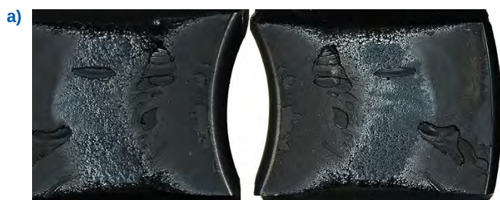
Figure 11: (a) Digital macro-photography image of full fracture surface of butt fused Sample 4 Specimen 3.
