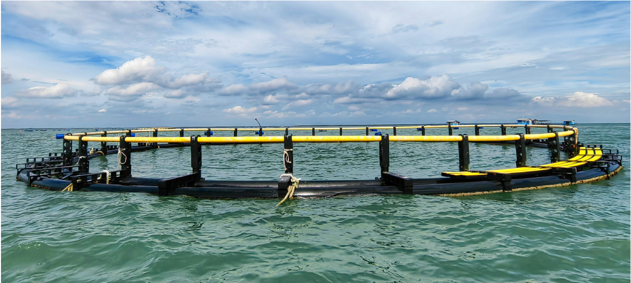
Spirolite's 19m diameter floating marine cage along the Malaysian Coast (Photo courtesy of Spirolite (M) Sdn Bhd)
