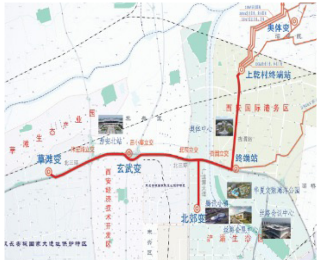
Connecting the double-circuit lines of 750kV Jingwei substation to 330kV Xuanwu substation, as well as the third circuit of 750kV Jingwei substation to 330kV Beijiao substation.
